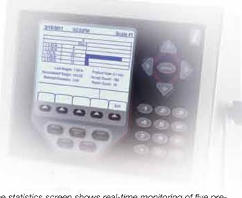
The statistics screen shows real-time monitoring of five preprogrammed weight zones, both per unit and cumulatively, illustrating where product falls within a targeted weight range.
